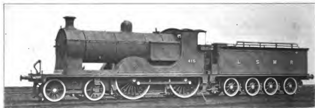
Fig. 5047. Eight-Wheel, Four-Coupled Locomotive. London & South Western. Cylinders 19 in. x 26 in.; Working Steam Pressure 175 lbs. per sq. in.; Total Heating Surface 1,550 lbs.; Diameter of Drivers 79 in.
